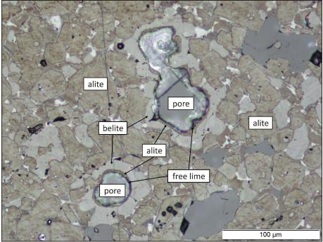
Figure 1: Two concentric structures of (from the inside out) pore, free lime, alite and belite, surrounded by a normal, alite-rich, microstructure.
