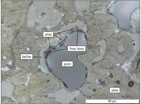
Figure 2: Concentric structure of (from the inside out) pore, free lime, alite and belite, surrounded by a normal, alite-rich, microstructure.
